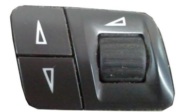
Track Down Volume Down
